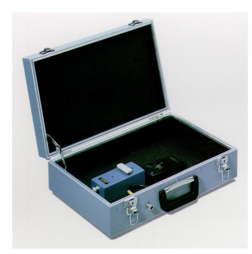
The shielded chamber of CTD-Z10 provides sufficient space for accommodating all customary analog and digital mobile phones. The antenna of the phone to be tested is connected to the coupler via a spring clamp. To achieve reproducible results, the coupler can be fixed to the chamber base. The radiospecific attenuation factors can be determined through calibration.
